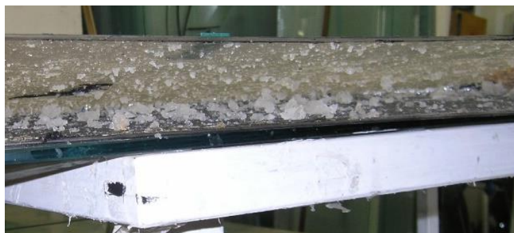
Figure 6. Soft siloxane clusters can be collected easily and recycled into silicone rubber.
