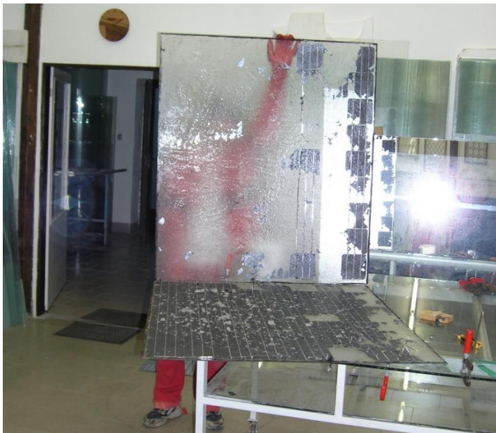
Figure 5. Separating nondamaged glass sheets with the remaining siloxane gel.
