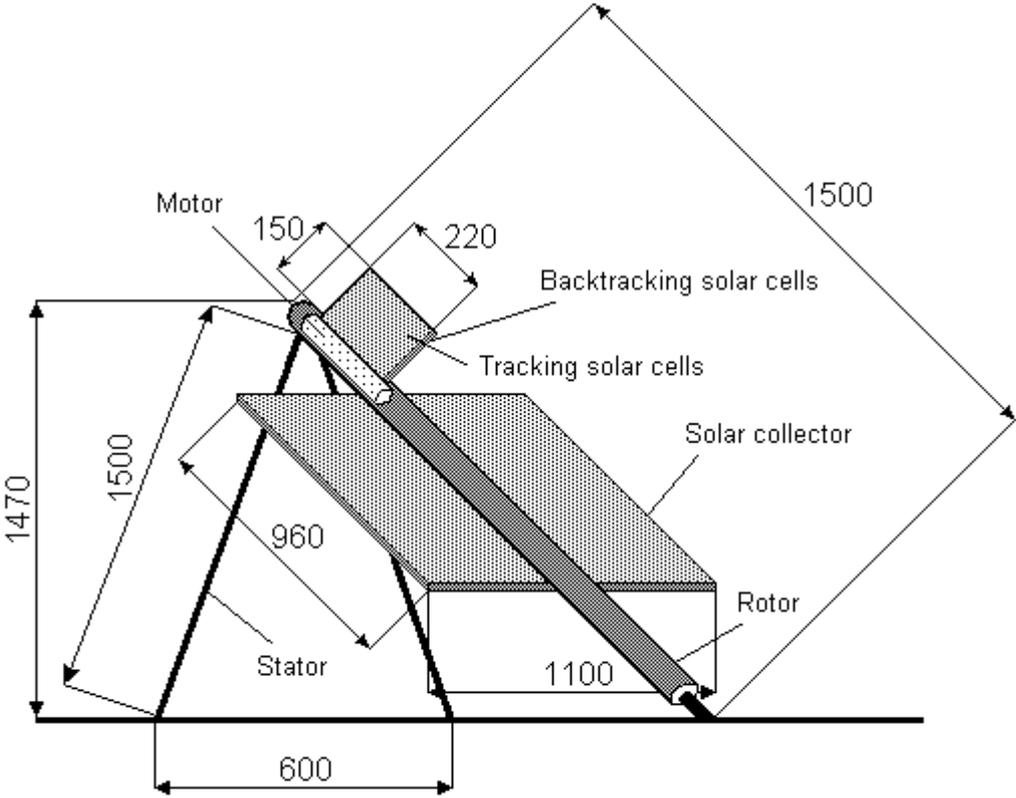
Fig.1 : The dimensional diagram of our tested device.
