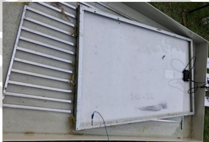
Fig 2. Photograph of the actual laboratory installation with the PP tank, immersed module and insulation tester.
