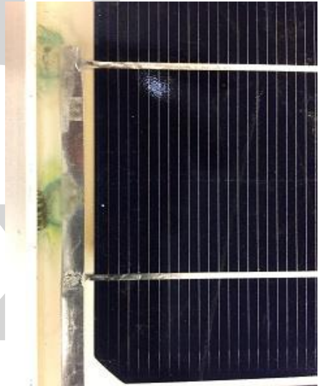
Fig. 5. Detail of another discharge channel
