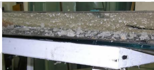
Fig. 4. Soft siloxane clusters can be easily collected and recycled into silicone rubber
