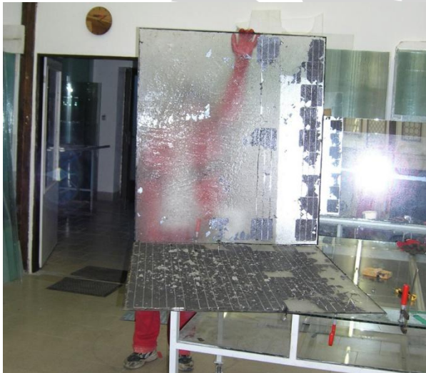
Fig. 3. Separation of non-damaged glass sheets with the remaining siloxane gel clusters.
